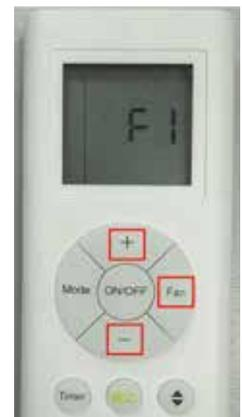
Use '+' and '-' to select E9, and then use 'MODE' button to enter into parameter selecting interface.
