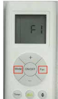
Use '+' and '-' to select 'd4', press 'FAN' button to send the confirm signal to the unit, the unit will enter into air flow test mode, and runs for 3~6 mins, then it will get the duct resistance.
