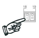
With the switch at I, the burner is powered electrically and is set up to run at request of the heating controller.
